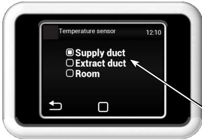
You can choose the output temperature sensor to control the unit.
