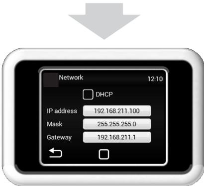
The NETWORK is used to set the unit's network communication (ModBus TCP)
