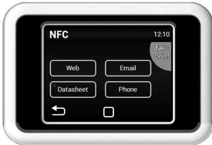
In the NFC menu you can display the information after placing an NFC compatible mobile device.
