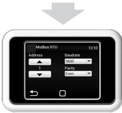
The MODBUS menu is used to set the Modbus communication.
